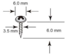
Do not drive the screws in all the way—leave a space of about 2 mm to allow room for sliding the wall-mounting panel between the wall and the screws.
