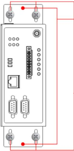
**Step 1:** Remove the aluminum DIN-rail attachment plate from the NPort, and then attach the wall-mounting plates with M3 screws.
